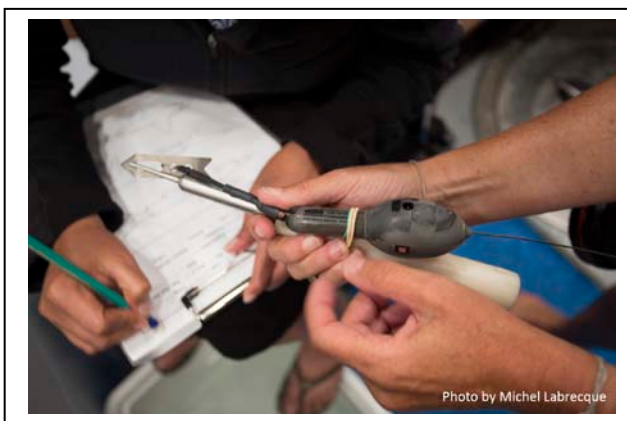
The specially designed tool used to attach the satellite tags to the shark's dorsal fin.
